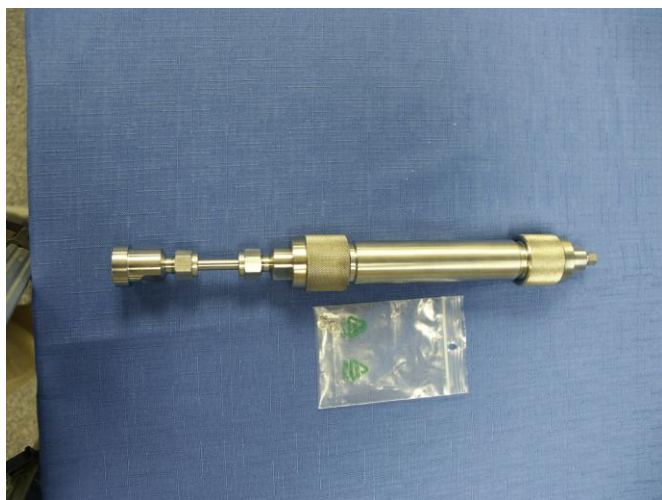
A 20ml Reservoir with all required fittings and pre-column for the 2.1mm X 15cm columns is included
